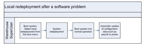
Figure 4-7 Process for local redeployment
